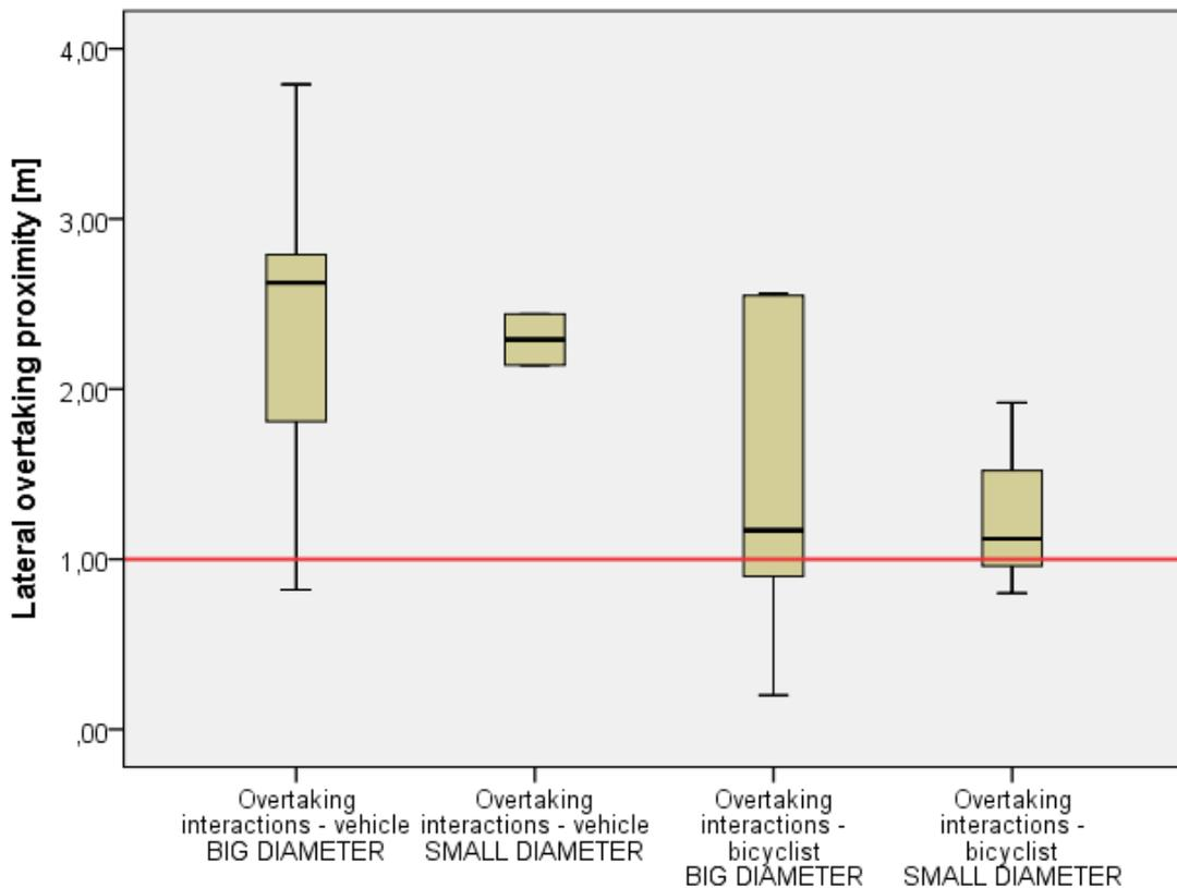
Figure 6 – Lateral overtaking proximity position of bicyclists for interactions 4 (*overtaking interactions – vehicle*) and for interactions 5 (*overtaking interactions – bicyclist*) for roundabouts with big diameter (30-32 m) and small diameter (20-22 m).
