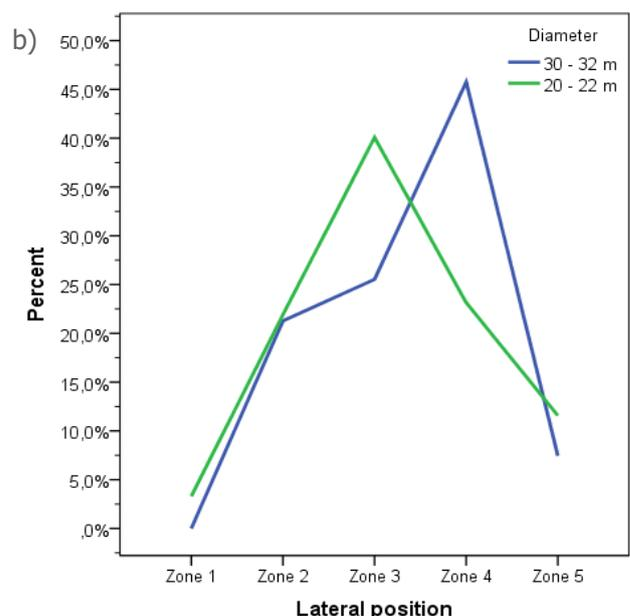
Figure 3 – a) Speed range of free-flow bicyclists for roundabouts with big diameter (30-32 m) and small diameter (20-22 m); b) Lateral position of free-flow bicyclists for roundabouts with big diameter (30-32 m) and small diameter (20-22 m).
