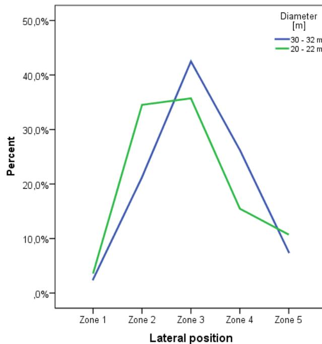
Figure 5 – Lateral position of bicyclists for interactions 2 (*following interactions – vehicle*) for roundabouts with big diameter (30-32 m) and small diameter (20-22 m).
